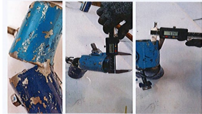
Figure 27. Measurement on Sleeve Coupler
