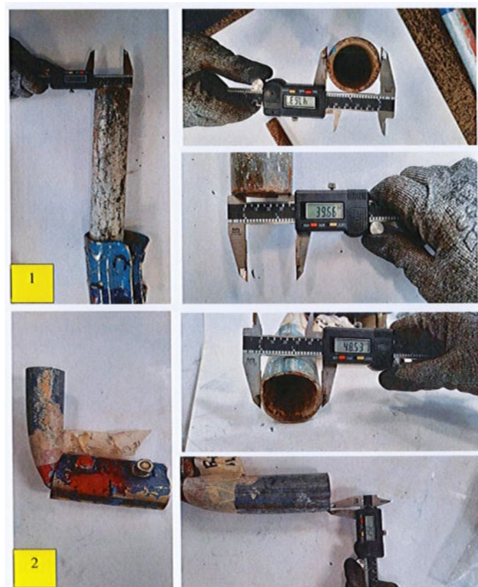
Figure 24. Measurement of Extender Tube
