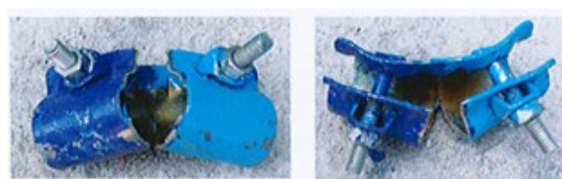
Figure 10. Damage of sleeve coupler
