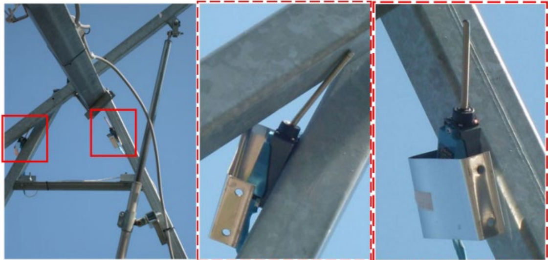
Figure 3. Location of end sensors of the system [10]
